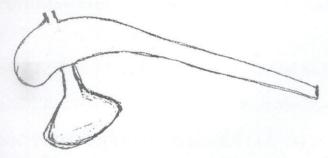
NAHUN (PUNGHUT): A tool like TOK use by carpenter. It is used in making boles of mirdanga.
